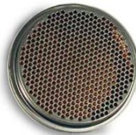
**Figure 3-2 The sonar transducer used in the robot**
